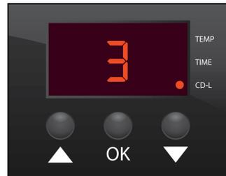
A red dot will appear next to "CD-L" when the press is closed. This indicates that the timer has started and is now counting down.
