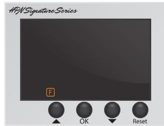
Press "OK". Use "▲" or "▼" to switch between "C°" or "F°" for your desired reading.
