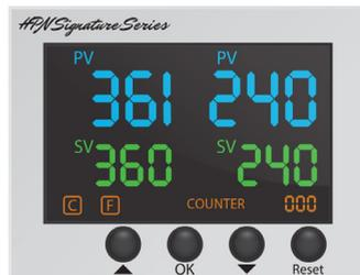
The "COUNTER" on the bottom right shows the number of transfer cycles. It can range from 0 to 999. Press "Reset" for 5 seconds to make counter go to 0.
