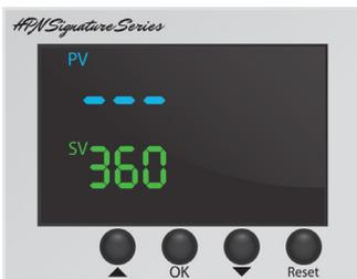
Press "OK" to set the temperature as labeled "SV". Use the arrow keys to select desired temperature.
