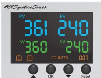
Press "OK" to enter real time mode. Note that "PV" is short for present value. "SV" is the desired value.
