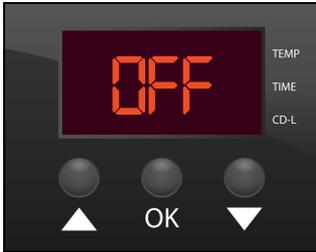
Turn on the power switch. It will say OFF. Press OK to turn on the machine. This is a safety feature.
