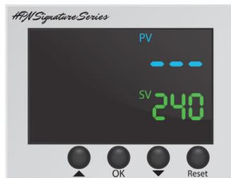
Press "OK" button to set time. This will be labeled "SV" on the right. Use arrow keys to set desired time.
