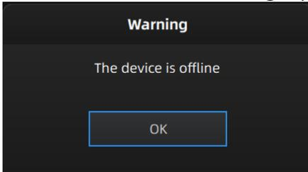
close the software by clicking the **X** in the upper-right corner of the screen. Verify the scanner has been turned on and try starting the software once again.
