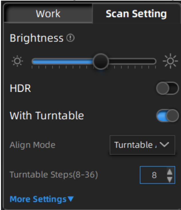
There are a couple of items to note on this screen. The brightness scale can be adjusted for room lighting and object texture. To scan an object with a high contrasting texture, such as something white and black, use HDR instead. If the object displays a large amount of red in the camera view, adjust the brightness scale accordingly so that a minimum amount of red is visible.
